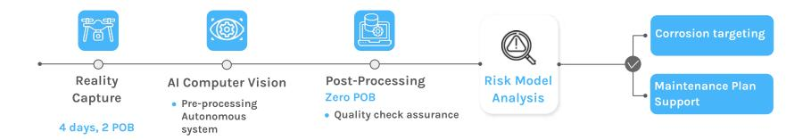
The solution combines reality capture via drone images in a 3D environment with Artificial Intelligence to view, locate, classify and quantify potential discontinuities, pitting and critical corrosion points.
